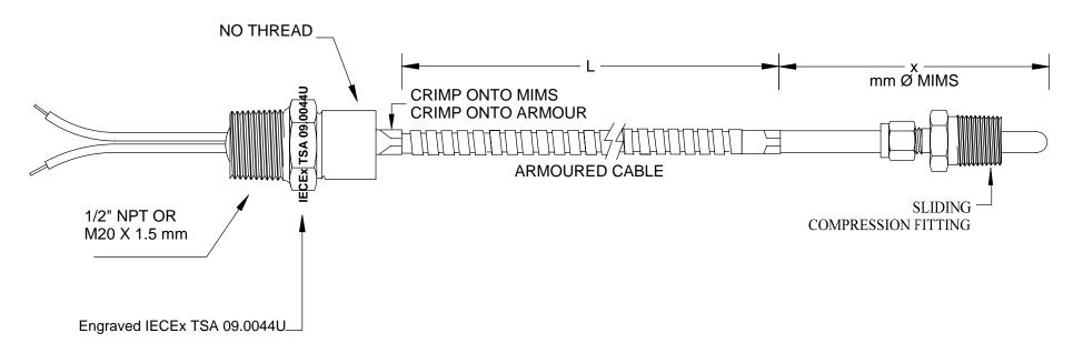
SUITABLE FOR USE WITH CERTIFIED Ex d / Ex e / Ex tD ENCLOSURE OR TRANSMITTER HOUSING WHICH HAS 1/2" NPT OR M20 X 1.5 MM PROCESS CONNECTION
